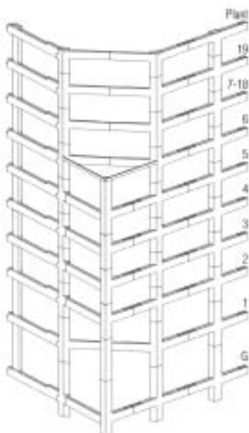
Precast cruciform beam and column layout
